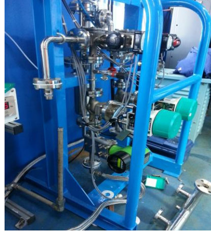
Ship ballast water system device
